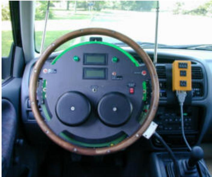
Figure 1.7: ATI/Heitz Sprint 3 steering controller
