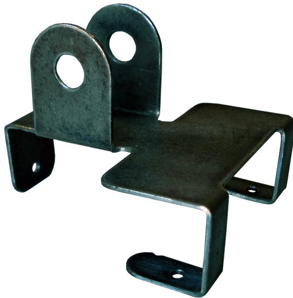
Figure 3.6: Clutch and brake pedals attachment
